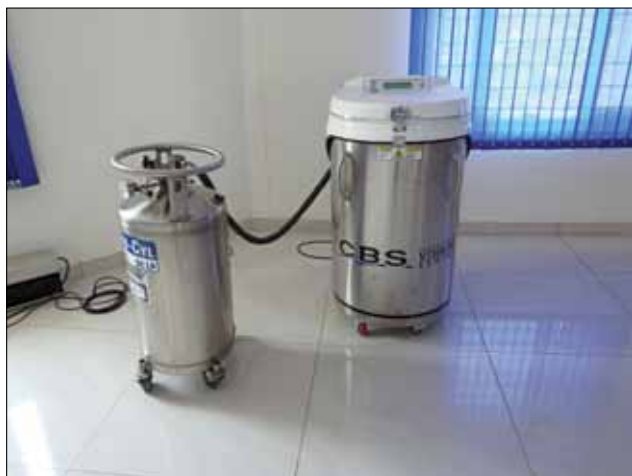
Fig. 80 Large scale storage of Indian major carp milt in Liquid nitrogen vapour phase storage system.
